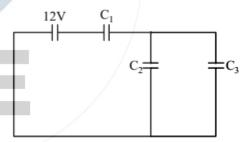
Now, C<sub>eq</sub> and C<sub>1</sub> are in series. Therefore, their equivalent capacitance is
