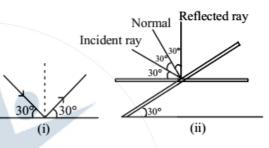
In order to make the reflected ray vertical, the mirror should be rotated at an angle of 60°.
