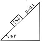
If  $\vec{F}_1$  is the force required to just move the block up the inclined plane and  $\vec{F}_2$  is the force required to just prevent the block from sliding down, then the value of  $|\vec{F}_1| - |\vec{F}_2|$  is : [Use  $g = 10m / s^2$ ]
