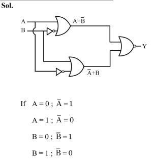
$$Y = \overline{\left(A + \overline{B}\right) + \left(\overline{A} + B\right)} = \overline{\left(1 + 1\right)} = 0$$
