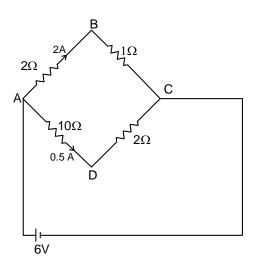
In steady state the capacitors will act as the open wire. Hence the circuit will be as above. If  $V_c = 0V$  then the potential at points A, B, C and D will be
