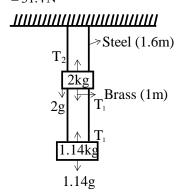
Elongation in steel wire  $\Delta L = \frac{T_2 L}{Ay}$
