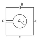
As shown in the figure, a single conducting wire is bent to form a loop in the form of a circle of radius r concentrically inside a square of side a, where  $a:r=8:\pi$ . A battery B drives a current through the wire. If the battery B and the gap G are of negligible sizes, determine the strength of magnetic field at the common centre O.
