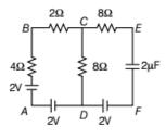
: In steady state, the combination of resistance and capacitance in loop CEFD will not work. So, we can eliminate this combination and hence the equivalent circuit is as shown below.
