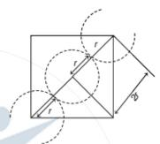
From the above figure, it is clear that the closest distance between two Au-atoms = 2r
