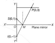
*I* is image of source *S* by the plane mirror placed perpendicularly along *X*-axis. SM = IM
