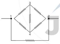
It is circuit of Wheatstone the equivalent resistance of upper circuit
