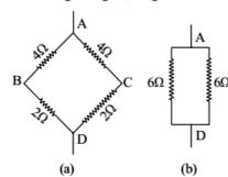
The  $4\Omega$  and  $2\Omega$  resistors are in series and the same is the case with another  $4\Omega$  and  $2\Omega$  resistors. So, the four resistors are equivalent to following two resistors.
