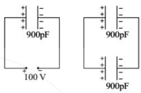
Q= CV= $(900 \times 10^{-12} \, \text{F}) \times 100 \, \text{V} = 9 \times 10^{-8} \, \text{C}$ When the battery is replaced by another capacitor of 900 pF capacitance, the charge of  $9 \times 10^{-8} \, \text{C}$  is distributed on both. Let  $Q_1$  and  $Q_2$  be the charge on each of them.
