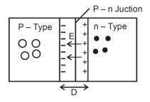
$$E = \frac{V}{d} = \frac{Potential\ barrier\ Across\ Junction}{width\ of\ Depletion\ layer}$$
