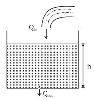
Since height of water column is constant therefore, water inflow rate (Qin) = water outflow rate
