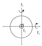
$I_1 + I_2 + I_3$  (Perpendicular axis theorem)
