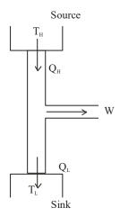
$$1 - \frac{Q_{L}}{Q_{H}} = 1 - \frac{T_{L}}{T_{H}}$$
